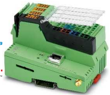
Entegre GSM/GPRS modemli
