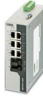
6 RJ45 port ve 2 fiber optik port (single mode)
